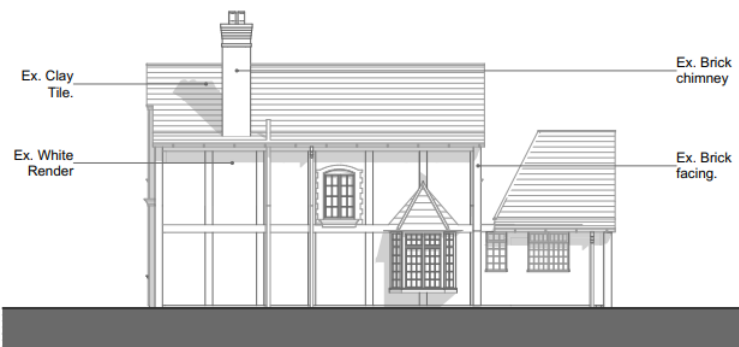
Existing East Elevations
