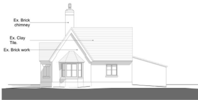
Existing East Elevation
